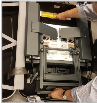
Fig. 12. Traveller's Conservation Copy Stand stowed in its suitcase.
