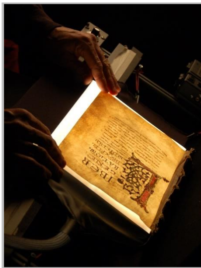
Fig. 22. Setup with infrared radiation used to capture watermarks.
