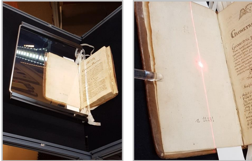
Figs. 6 and 7. Tools to hold down folios: an acrylic plate and an acrylic finger. 65
